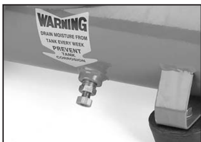
Figure 10. Tank drain valve.
